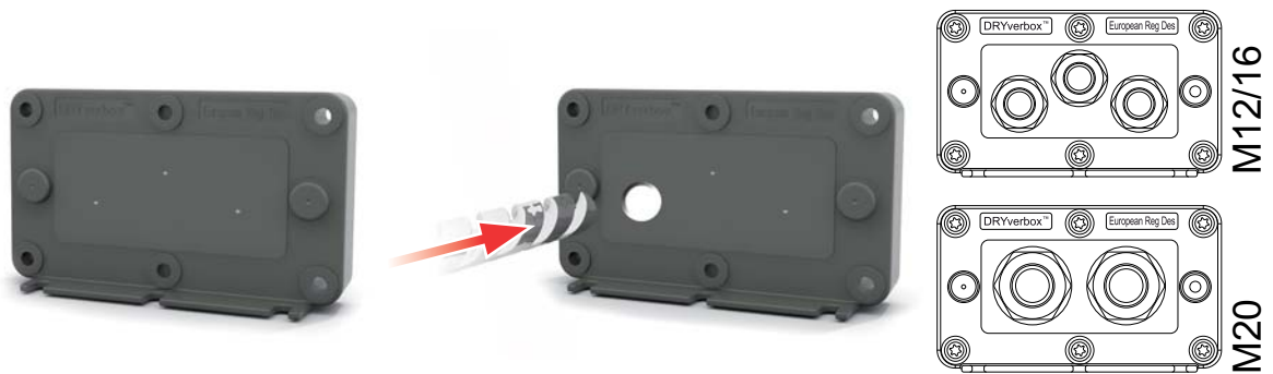
D Drilling holes for the glands: M12 (max 3), M16 (max 3) or M20 (max 2)
