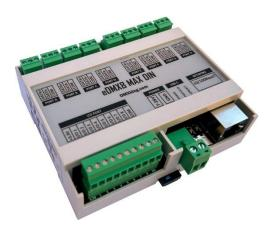
Network 10/100Mbps RJ45 socket. Pluggable 2way 5mm pitch terminal block for 7-28Vdc power input. Eight 3way 3.5mm pitch pluggable terminal block connectors for DMX512.
